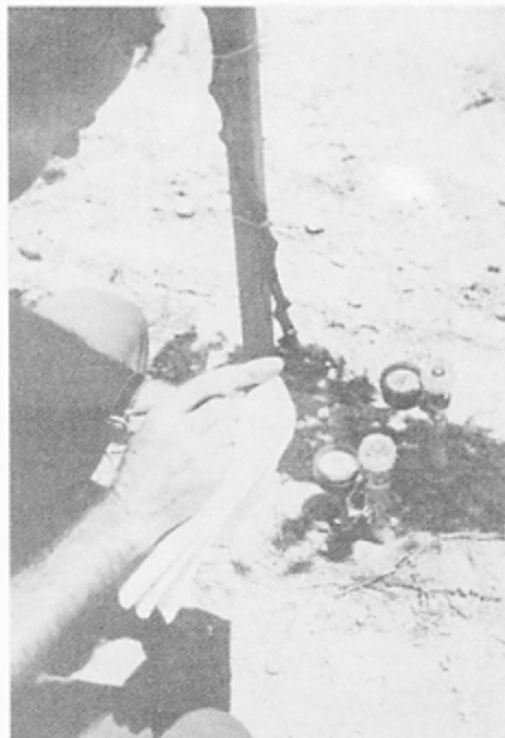
JOHN MORAMARCO takes a moisture reading on one of the many Irrometer stations at La Serena Vineyards Association. These devices take the guesswork out of timing irrigations.
