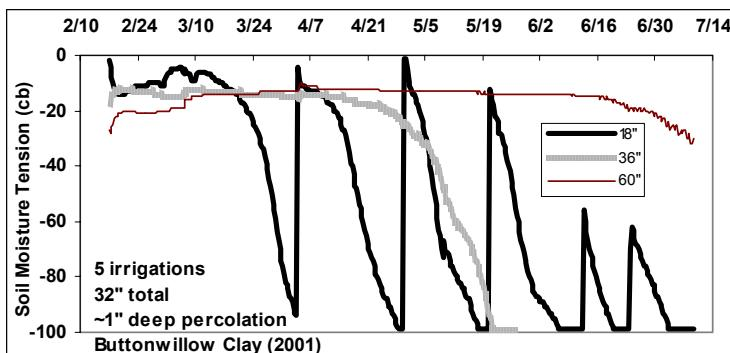
Fig. 8. Soil moisture “tension” changes during the 2001 season for beets in Buttonwillow Clay and irrigation intervals of approximately 3 weeks. This field is adjacent to the 2002 Buttonwillow Clay field.
