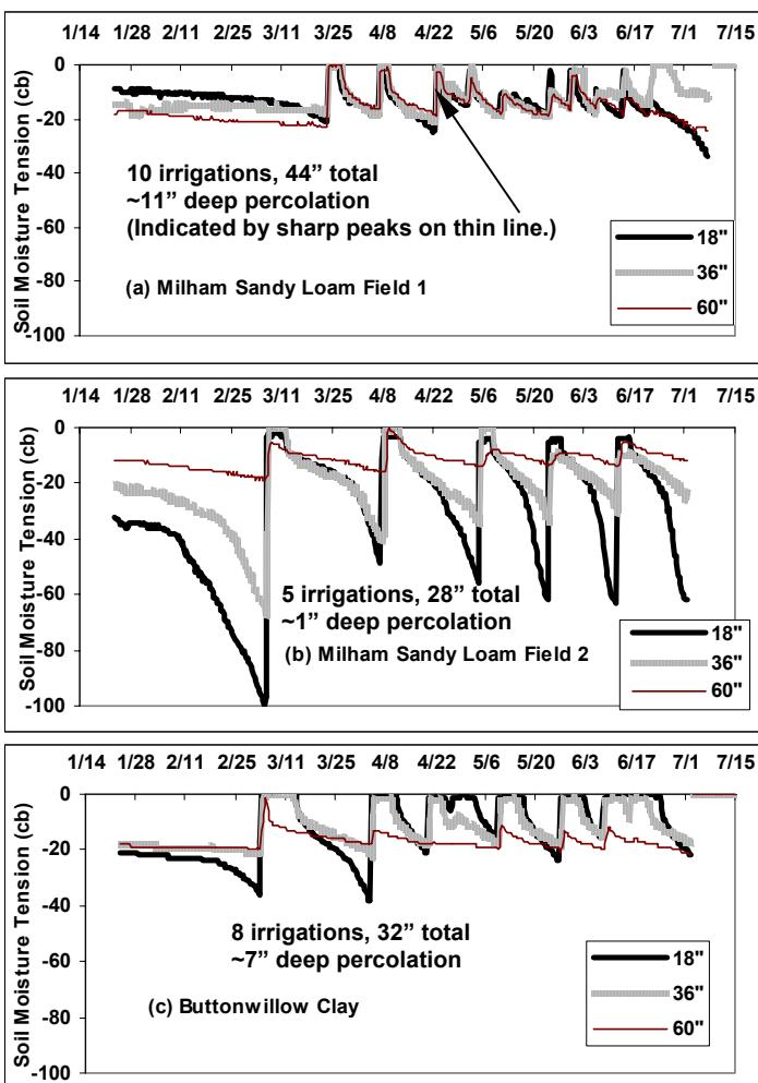
Fig. 7. Soil moisture “tension” changes during the 2002 season as measured by Watermark electrical resistance sensors and recorded every 8 hours with the AM400 data logger.
