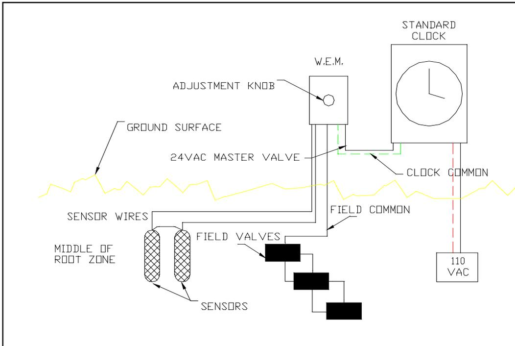
**Figure 1: Sensor Installation**
