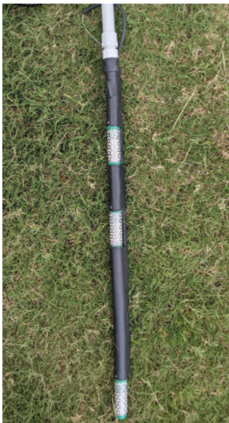
Figure 1. Probe containing three soil water tension sensors.
